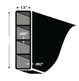
We crimp or notch both sides on both ends to secure the rail into the post. The triple-rib rail design provides extra impact resistance while maintaining flexibility for the safety of your horses.
