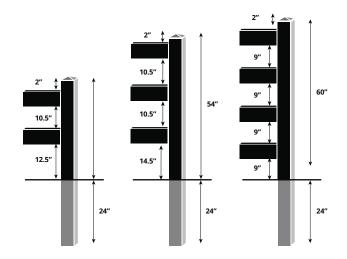
Rails are 16' long and designed to alternate between posts to increase strength. Posts are placed on 8' centers. **Call for more information on spacing and sizes.**
